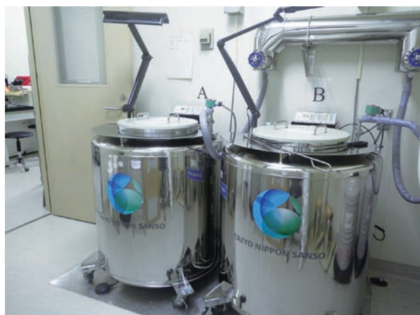
Figure 4. Liquid nitrogen tank
