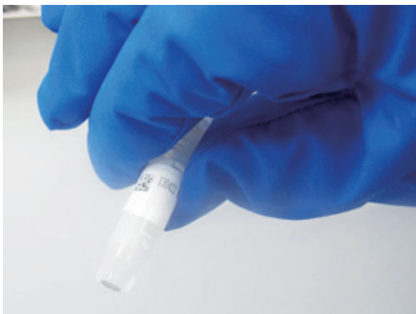
Figure 3. Cryo tube with 2D barcode. Each sample is printed with a unique barcode and is managed using a database.
