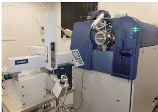
Figure 2. Triple TOF LC/MS/MS System
