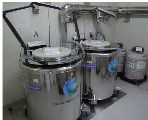
Figure 4. Liquid nitrogen tank.
