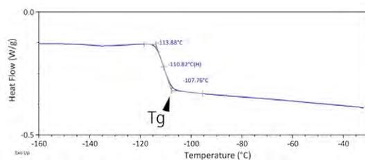
Figure 2. Differential Scanning Calorimetry (DSC) thermogram of Vitrified shoot apices of a Chrysanthemum plant treated with vitrification solution.
