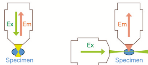
Figure 2. Principle of light-sheet microscopy. Left: light path of conventional fluorescent microscopes using single objective lens for both illumination (Ex) and detection (Em). Right: light-sheet microscopes including DSLM, where illumination light is limited to the focal plane of the detection objective.
