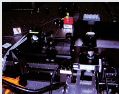
Optical path of the DSLM
