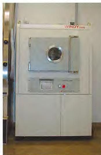
Figure 3. the animal radiation wastes drying system (Wakaida Engineering Co. type WINDY2000)
