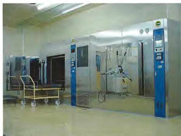
**Figure 2.** Autoclaves of a large scale for sterilization.
