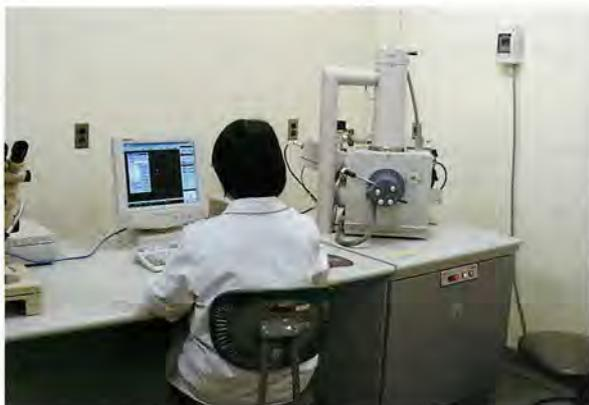
Figure 2. Environmental Scanning Electron Microscope.
