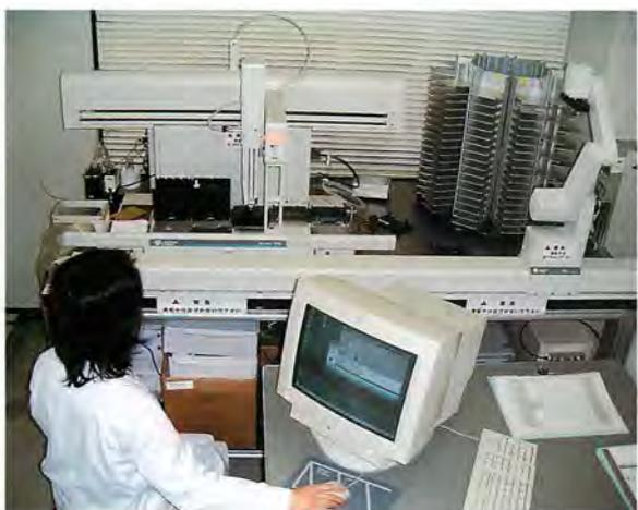
Figure 2. Biomek 2000 Laboratory Automation System.
