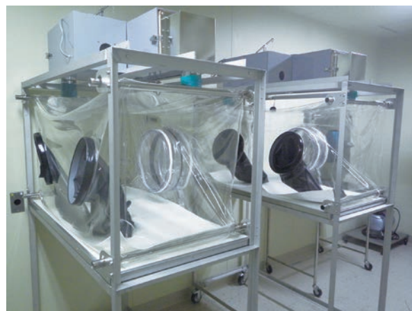
Figure 5. Vinyl isolators in the quarantine room
