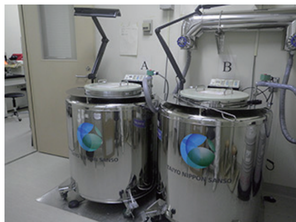
Figure 4. Liquid nitrogen tank.
