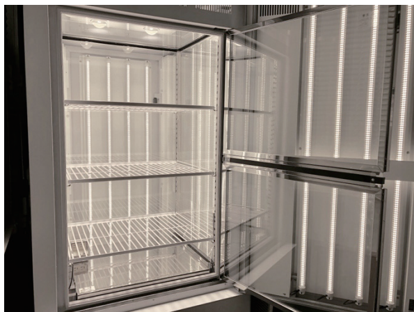
Figure 5. A plant culture box with high luminance LED lamps.
