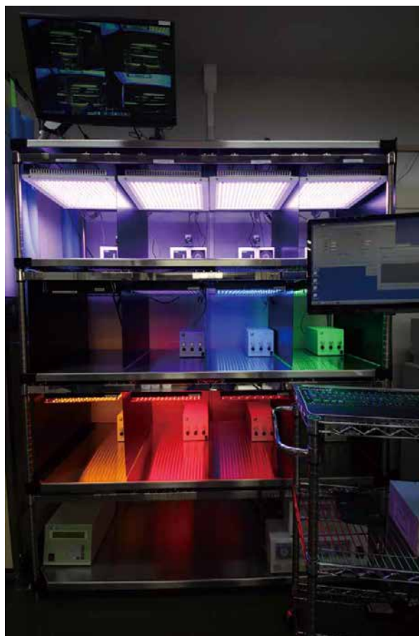
Figure 5. A tissue culture rack with dimming LEDs and pulse-width modulation controllers.
