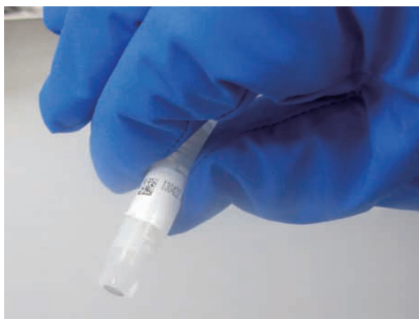
Figure 2. Cryo tube with 2D barcode. Each sample is printed with unique barcode and is managed using database.
