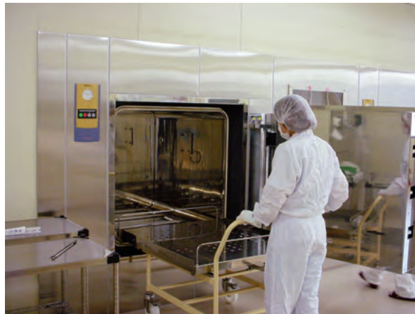
Figure 2. Large scale autoclaves for sterilization
