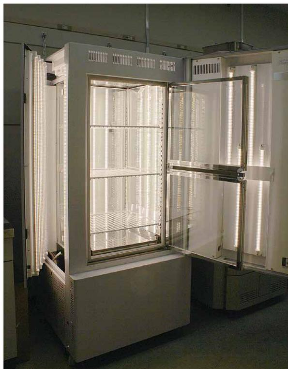
Figure 5. A plant culture box with LED lamps.
