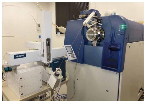
Figure 2. Triple TOF LC/MS/MS System
