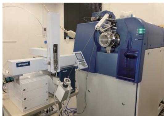
Figure 2. Triple TOF LC/MS/MS System
