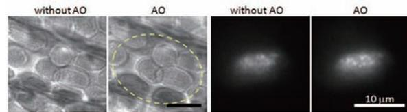
Figure 1. Effects of adaptive optics (AO) to wide-field microscope images (bright field and fluorescence of plant cells).
