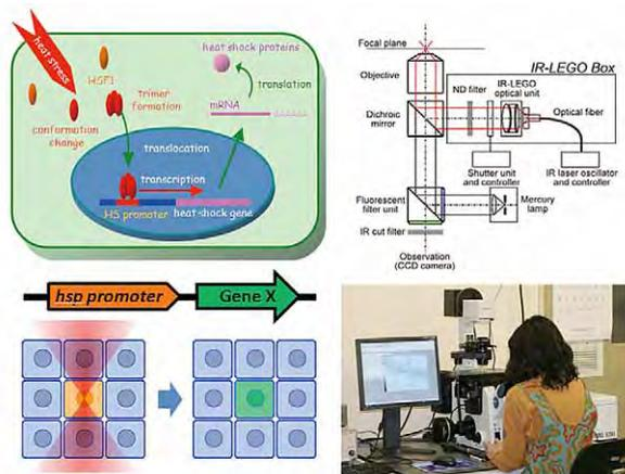
Figure 2. Schematic illustration of local gene induction system and an infrared laser-evoked gene operator (IR-LEGO) microscope system in NIBB.
